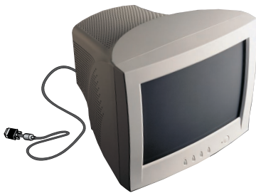
CRT Display with attached Video Cable
